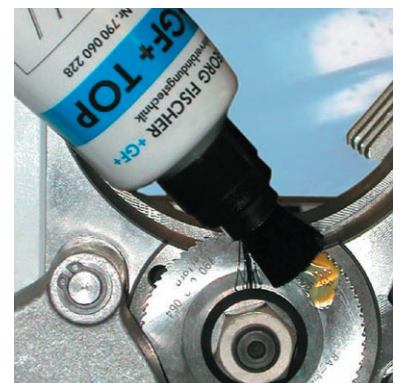
GF TOP is equipped with a little screw on brush to precisely apply the lubricant onto the tool.
